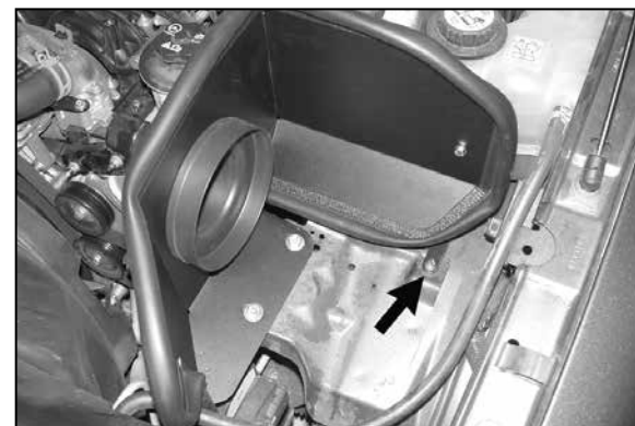
16. Install the heat shield into the vehicle and secure the "L" bracket to the threaded hole on the inner fender using the provided hardware as shown but do not tighten at this time. NOTE: Due to manufacture inconsistencies, some vehicles may not be equipped with threaded hole in the factory filter mounting plate. It will be necessary to drill a 1/8" hole in the air filter mounting plate and attach the heat shield bracket with the sheet metal screw provided.
