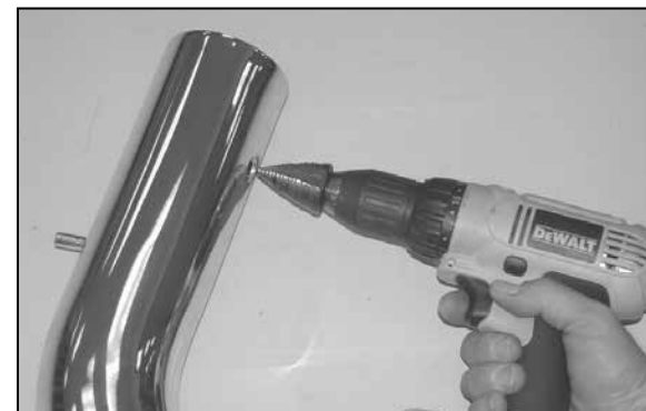
17b. Remove the intake tube and drill a 5/8" hole at the location marked in step #17a. NOTE: Be sure to remove all the burrs after drilling.
