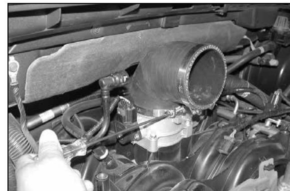
17. Install the 90° silicone hose and hose clamps onto the throttle body as shown but do not tighten completely at this time. NOTE: The hose has one short leg and one long leg, the short leg goes on the throttle body and the long leg goes to the intake tube.
