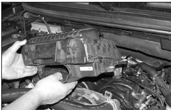
8. Pull firmly upwards to remove the air cleaner as shown. NOTE: K&N Engineering, Inc., recommends that customers do not discard factory air intake.
