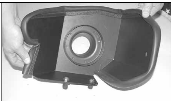
14. Install the provided trim seal onto the heat shield and trim to fit as shown.
