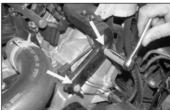
10. On vehicles equipped with the intake tube support bracket, reinstall the two nuts removed in step nine as shown.
