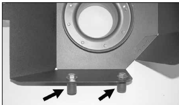
13. Install the provided rubber inserts, hex bolts and washers onto the heat shield as shown, but do not tighten at this time.
