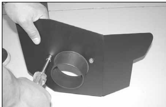
12. Apply the provided thread locker onto the provided hardware and secure the filter adapter onto the heat shield as shown.
