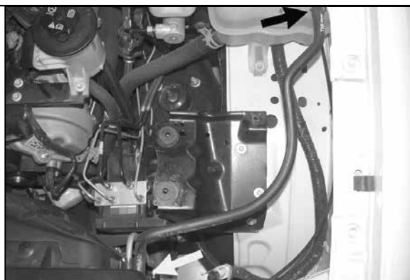
15a. Loosen the coolant recovery hose, hose clamps, and then remove the factory recovery hose shown. Be sure to catch any coolant, which flows out of the radiator during hose removal. NOTE: Be sure to let the engine cool completely before removing the overflow hose or hot coolant will escape from the radiator and injury or damage may result.
