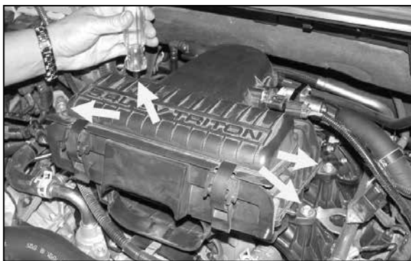
7. Remove the four bolts that secure the air cleaner as shown.
