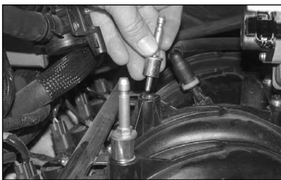
8a. Re-install the factory airbox mounting studs with the provided spacers as shown.
