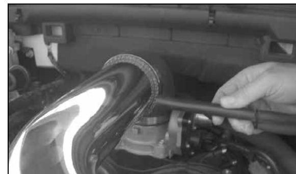
17a. On vehicles equipped with the brake booster vent line install the K&N® intake tube into the silicone hose at the throttle body. Align the brake booster vent line to the K&N® intake tube as shown and place a mark for drilling location.
