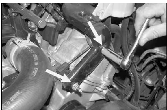
9. On vehicles equipped with the intake tube support bracket, remove the two nuts and then remove the stock intake tube support bracket as shown.
