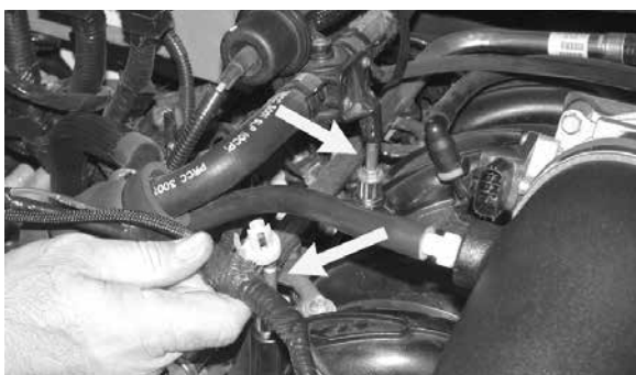
8b. Re-install the heater control valve and wiring harness mounting clips onto the airbox mounting studs as shown.
